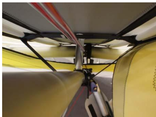
Figure 5-2 : Path of Tensioning Cables
