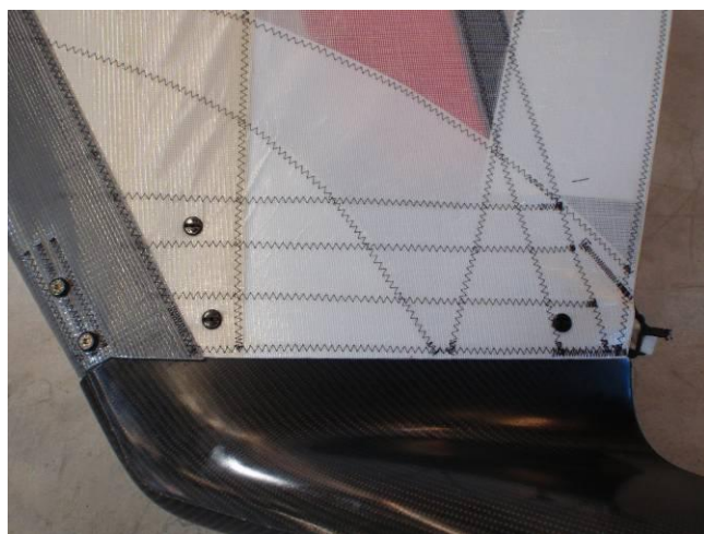
Figure 5-3 : Wing Tip Fin Fasteners
